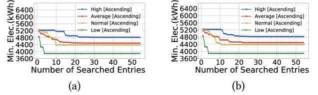
Figure 20: Under High, Normal, Average and Low cooling demands: minimum electricity consumption under the number of searched entries, ranked by (a) Electricity Consumption and (b) Cooling Load.
