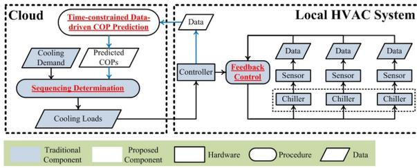
Figure 4: Framework of Data-driven Chiller Sequencing.
