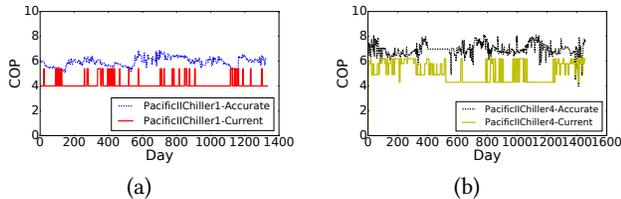
**Figure 16: The accurate COP and estimated COP with present scheme on different days in Pacific Place II for two types of chillers (a) Chiller 1; (b) Chiller 4.**
