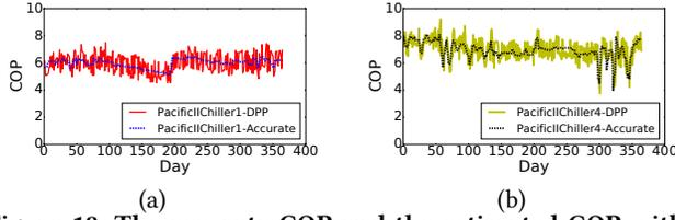
Figure 18: The accurate COP and the estimated COP with DPP scheme on different days in Pacific Place II for two types of chillers of (a) Chiller 1; (b) Chiller 4.
