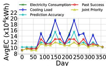
**Figure 21: The average electricity consumption ordering with different factors under days.**
