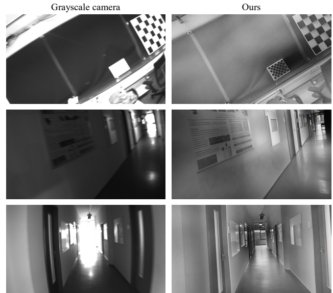
Fig. 5: Under HDR and fast motion conditions, grayscale camera images suffer from saturation and loss of details, whereas our diffusion-restored intensity observations preserve clear structure and stable contrast.
