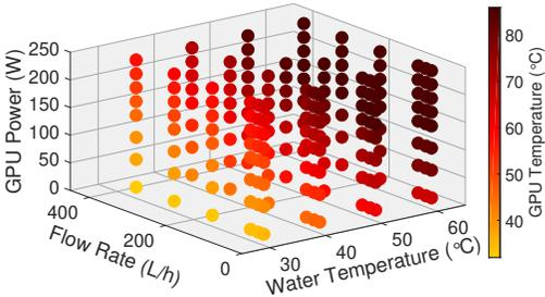
**Figure 10: Measurement results of GPU temperature with different inlet water temperature, water flow rate, and GPU power.**
