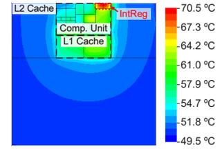
**Figure 2: Temperature distribution inside a CPU core.**
