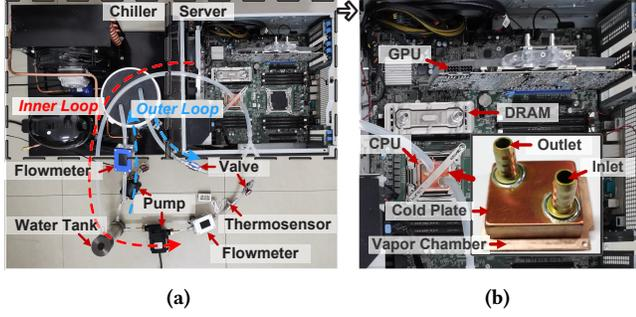
Figure 12: Hardware prototype of CoolEdge.
