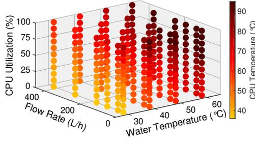
**Figure 9: Measurement results of CPU temperature with different inlet water temperature, water flow rate, and CPU utilization.**
