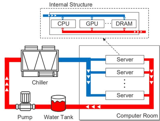
Figure 1: Water cooling architecture in an edge datacenter.
