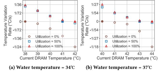
**Figure 11: DRAM temperature variation rate (the solid points represent the stable temperatures).**
