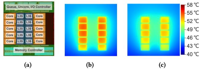
Figure 7: (a) The die shot of Intel Xeon E5 CPU [103], and thermogram of the die cooled by the (b) commonly used cold plate and (c) vapor chamber-based cold plate.
