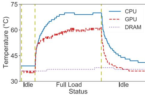
**Figure 3: Temperature variation of heterogeneous hardware components.**
